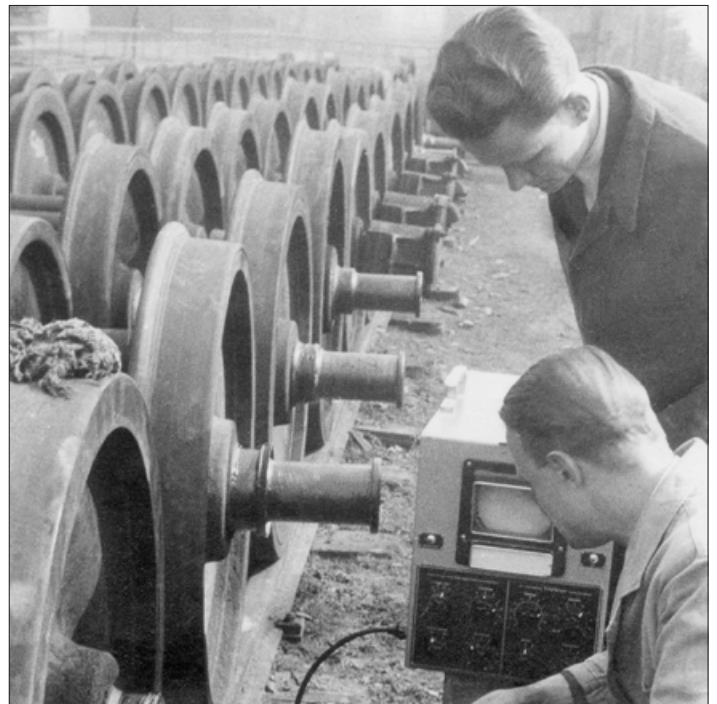
Volker Deutsch as a test engineer (top) with an early ECHOGRAPH ultrasonic testing instrument during his time as a doctoral student in Hanover
