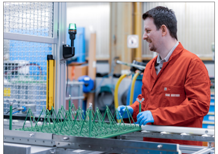
Output station with light barrier and trolley
