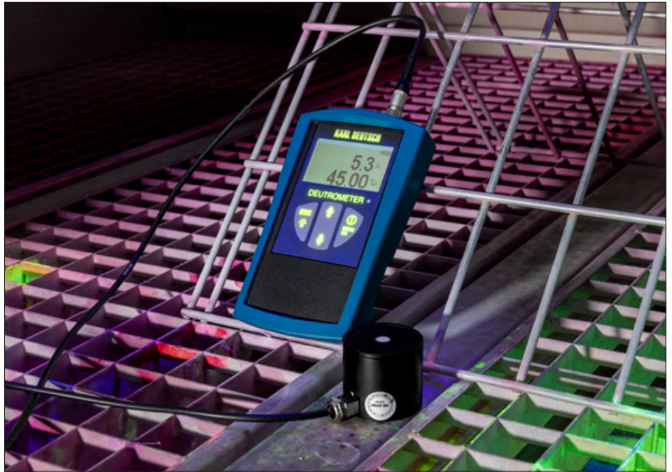
The DEUTROMETER is also the perfect tool for checking the illumination conditions during penetrant testing.
