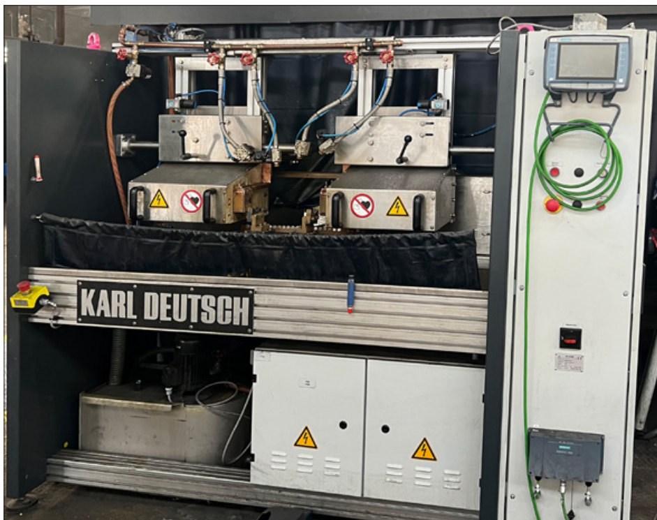
DEUTROFLUX UWE 600 with workpiece ejector and mobile control panel
