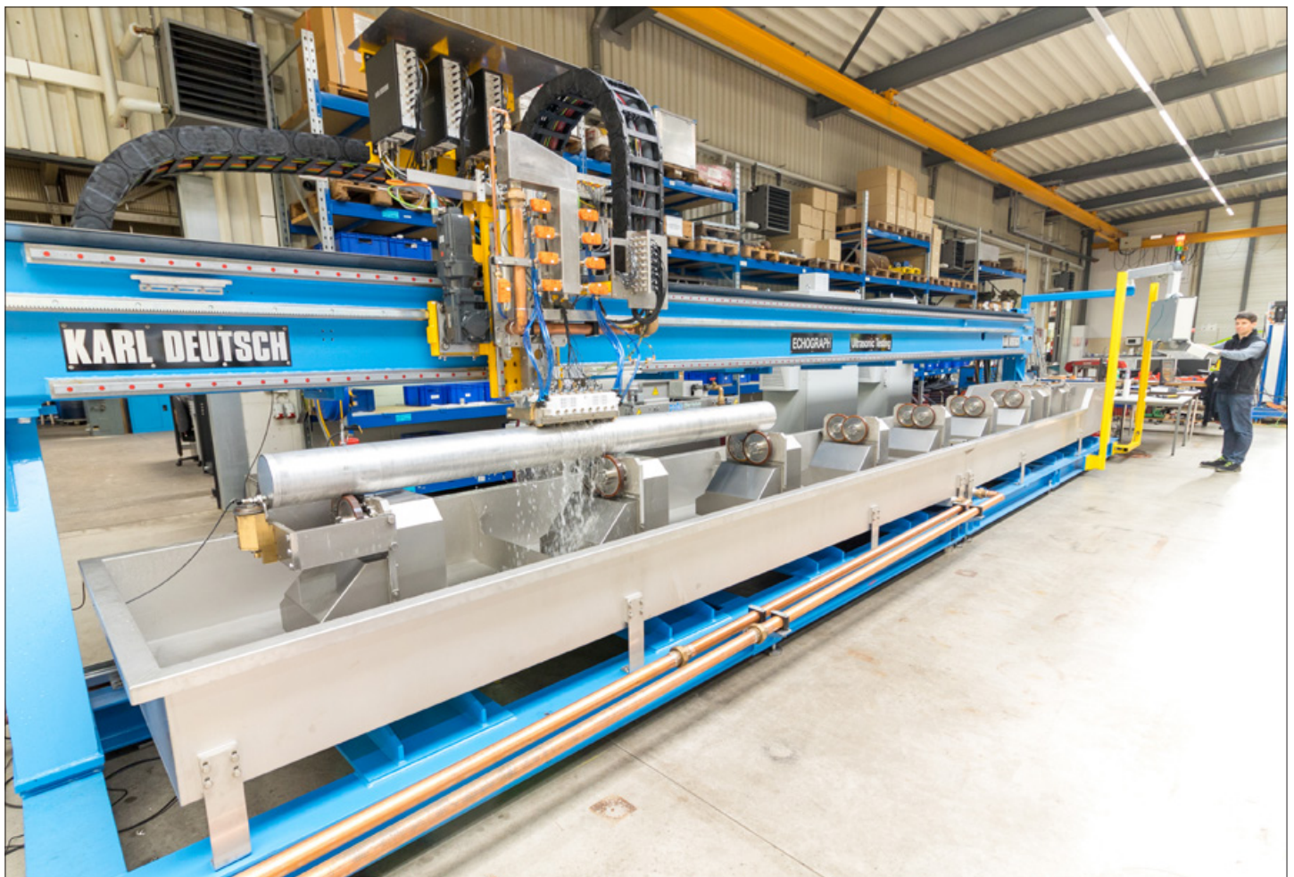
ECHOGRAPH RPTS system for testing aluminium bars before shipment at KARL DEUTSCH in Wuppertal
