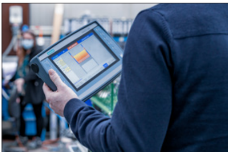
KD-CHECK MEMORY: Mobile panel for entering and monitoring test parameters
