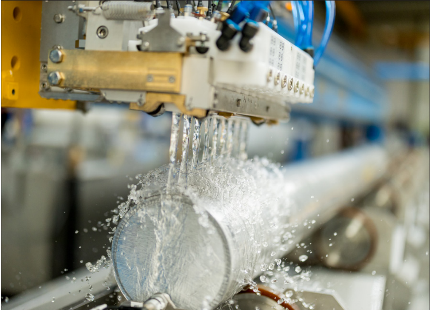
Squirter coupling for high testing sensitivity, quick changeover and long service life of the probes
